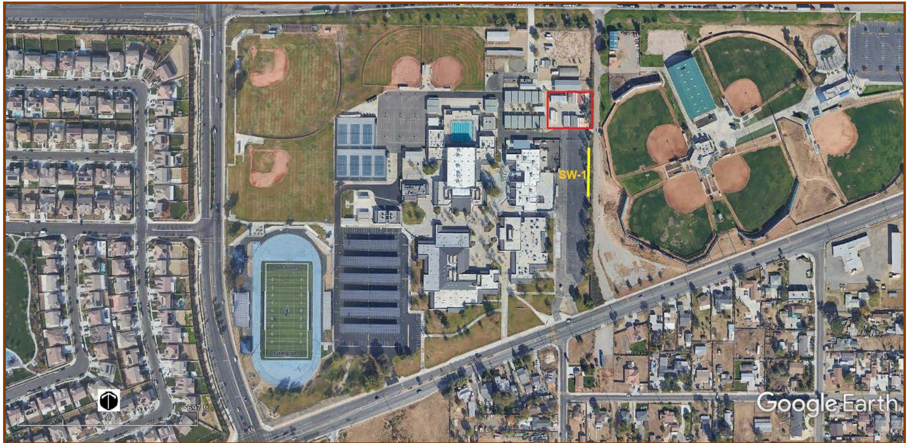
Base Map: Google™ Earth (2022); Project site area outlined in red; Seismic shear-wave survey line (SW-1) shown as yellow line.
